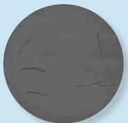
2 rating – Pass Less than 6 internal cracks, each shorter than 50% of the cross section, with a total crack length of less than 2.5 times the cross section.
