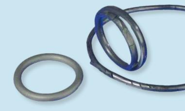
A comparison between FR68/90 and an alternative elastomer material following RGD testing illustrates the importance of selecting the correct material for applications prone to RGD.
